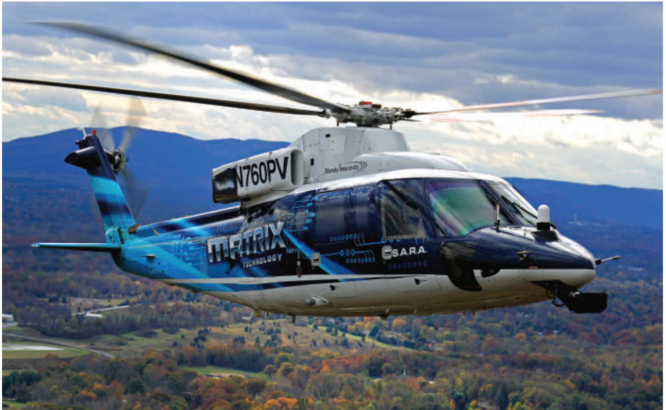
The Sikorsky Autonomous Research Aircraft, or SARA, is a modified S-76B helicopter using the Matrix Technology autonomy system.
