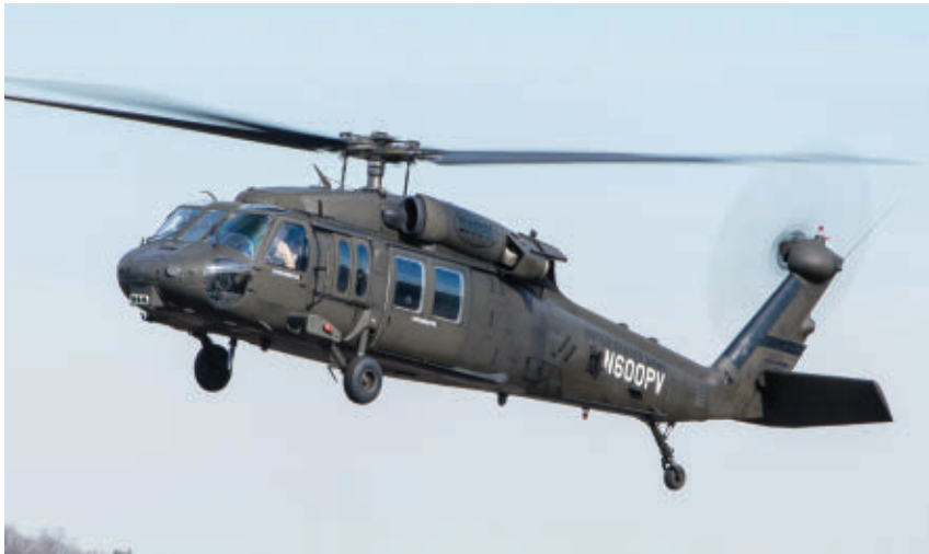
The modified Black Hawk helicopter S-70 Optionally Piloted Vehicle (OPV) Black Hawk has full-authority, fly-by-wire flight controls.
